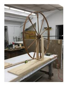
act as the axle for the wheel<sup>24</sup>. On the inside cavity of the drive wheel I placed a neoprene spacer to balance out the wheel with the axle adjacent to the original horn spacer. I glued caps to the sides of the support arms so that the axle would not slip and could only be removed from the top. I rounded the portions out
